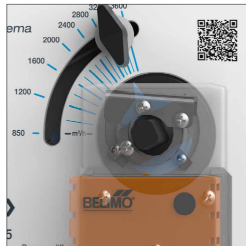
11. Unscrew the handle, press and hold the black button and set the indicator on the wanted maximum air flow value. In this case we will set it to the 2600 m 3 /h. Release the button and tighten the handle again
