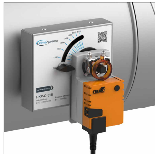
5. Lock lower part of the actuator on the motor mount and upper part on the motor shaft. The lateral side of actuator should be parallel with the lateral side of mechanism cover
