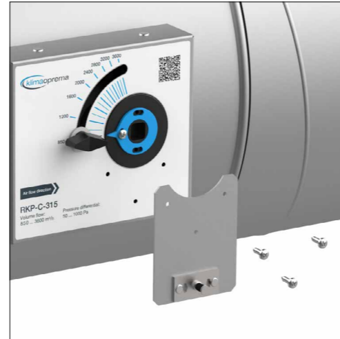
3. Pierce the product sticker on the X marks and install motor mount with three self-tapping screws; 3,9x13 DIN 7981.
