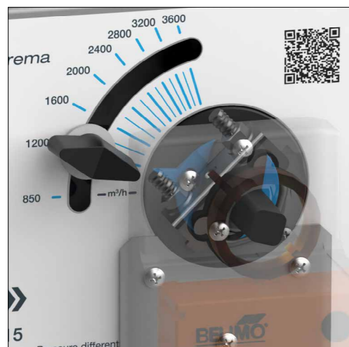
9. Unscrew the handle, press and hold the black button and set the indicator on the wanted minimal air flow value. In this case we will set it to the 1200 m³/h. Release the button and tighten the handle again
