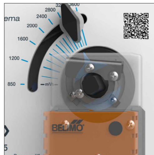
11. Unscrew the handle, press and hold the black button and set the indicator on the wanted maximum air flow value. In this case we will set it to the 2600 m³/h. Release the button and tighten the handle again
