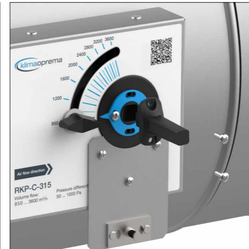
4. Install the motor shaft with two self-taping screws 3,9x13 DIN 7981. (1,5 Nm)
