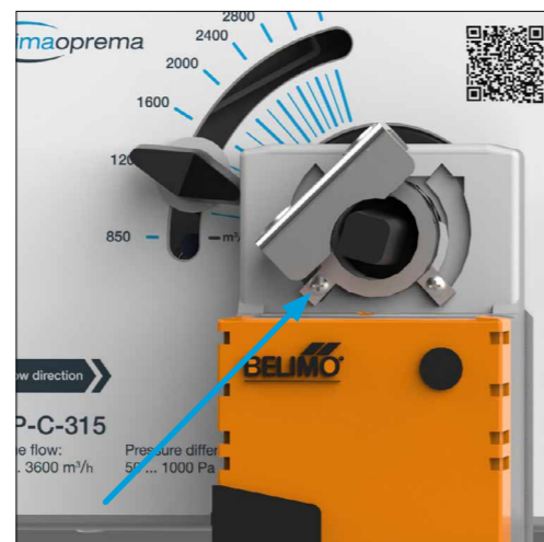
10. Unscrew the screw on the left limiter; push and tighten it under the jaw
