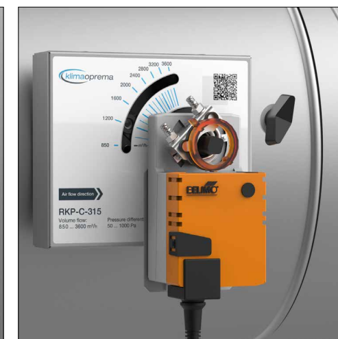
13. Unscrew the handle, press and hold the button, rotate the jaw together with shaft to the previously minimum set value and remove the handle at the end
